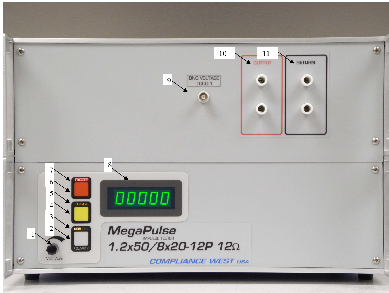
Figure 1. Controls, Indicators, Connectors – MegaPulse 1.2x50/8x20-12P 12 ohm Front Panel
